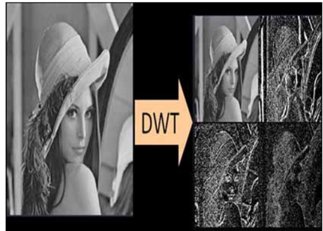
Fig. 6 Test Image is decomposed by DWT into four subbands
