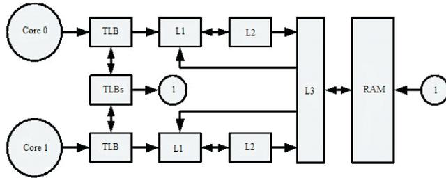
Fig.1. Memory hierarchy of the processor Intel i5-460M
