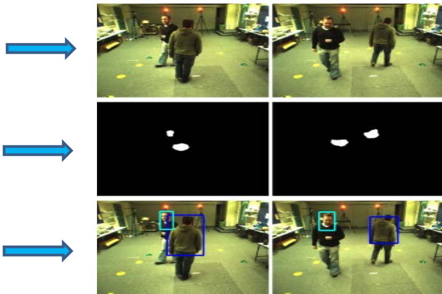
Fig.3 First row indicates the original image, Second row shows the segmented object and Third row shows the detected object.
