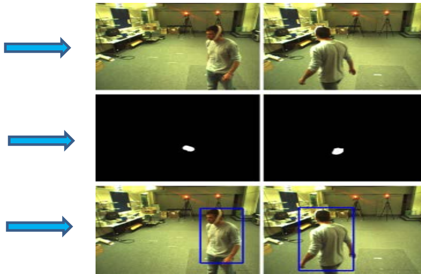
Fig.2 First row indicates the original image, Second row shows the segmented object and Third row shows the detected object.
