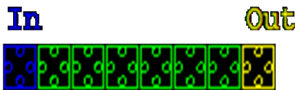
Fig. 4 QCA wire with 45 0 oriented QCA Cells
